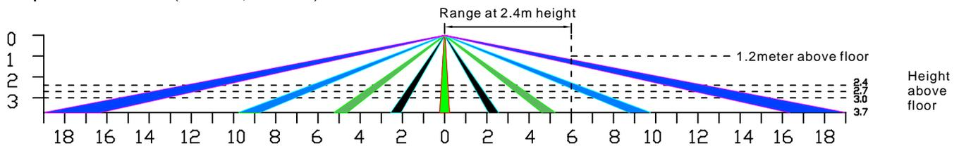
**Sensor Optical View Pattern** (top view, in meters, 2.4m mounting height)
